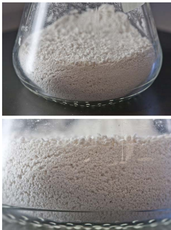
Figure 3. Example of a caked batch after achieving L/S_{\max} .
